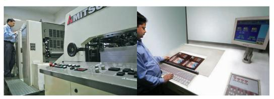
A dust-free air-conditioned environment complements our printing floor that has a wide array of printing presses – 1, 2 and 4 colour Heidelburg CP Ttronic and 5 colour Mitsubishi 1000 Series offset printing machines – in various sizes and configurations that can handle diverse print jobs.
